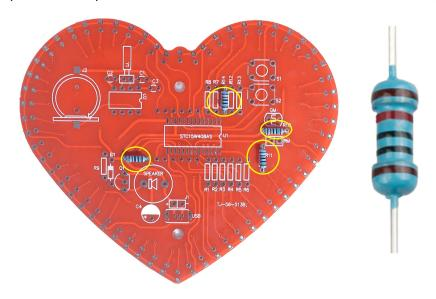
Step 2: Install 8pcs 330ohm Metal Film Resistor at R1-R8.
